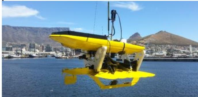
*Wave Glider being prepared to be loaded onto ice breaker ship to head to Southern Ocean*
